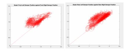
• Relationship between the Damper Positions on the left and the right side agwith respect to time
